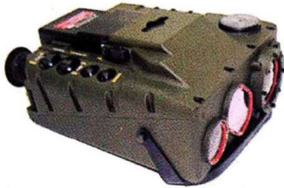
Figure 1-1: HHTI with LRF
